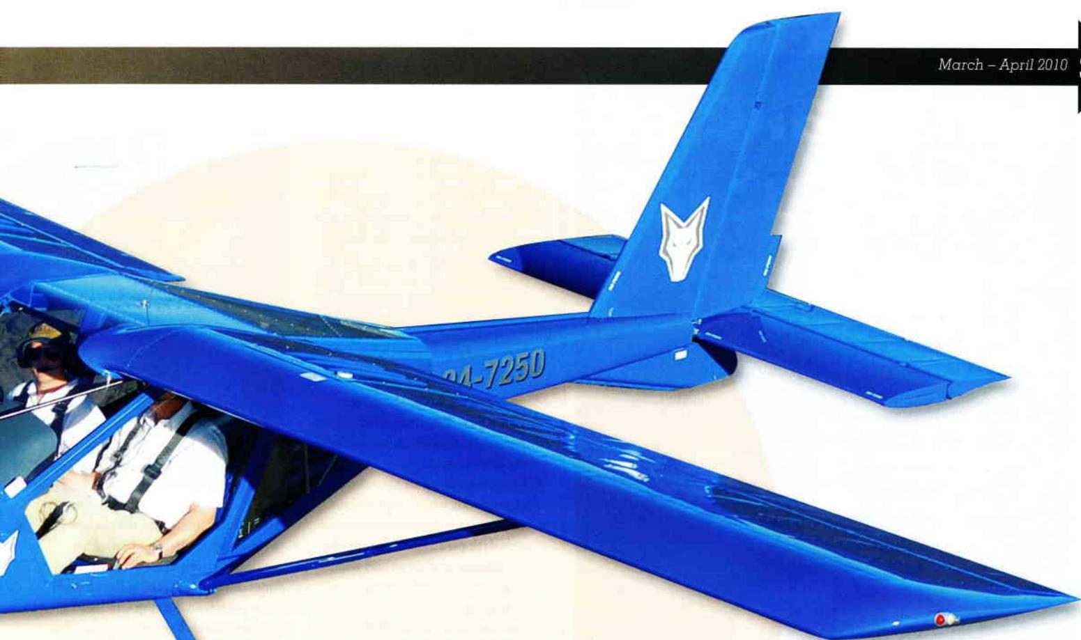
"To keep the centre of gravity (CoG) where it should be, it was decided to sweep the wings forward slightly.
