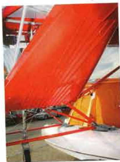
The tail unit consists of a big sweptback fin, small ventral fin, large rudder and single-piece elevator. Note the small wheel at the base of the ventral fin.
