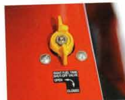
The dual fuel valves are above and behind your head. They really should be in front of you.
