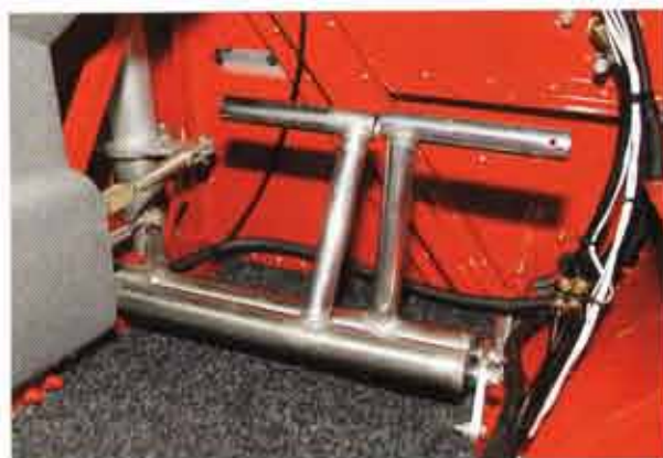
Below Right: The centre console contains levers for the throttle, brake, trim and water rudders. The large lever releases the undercarriage's uplocks.
