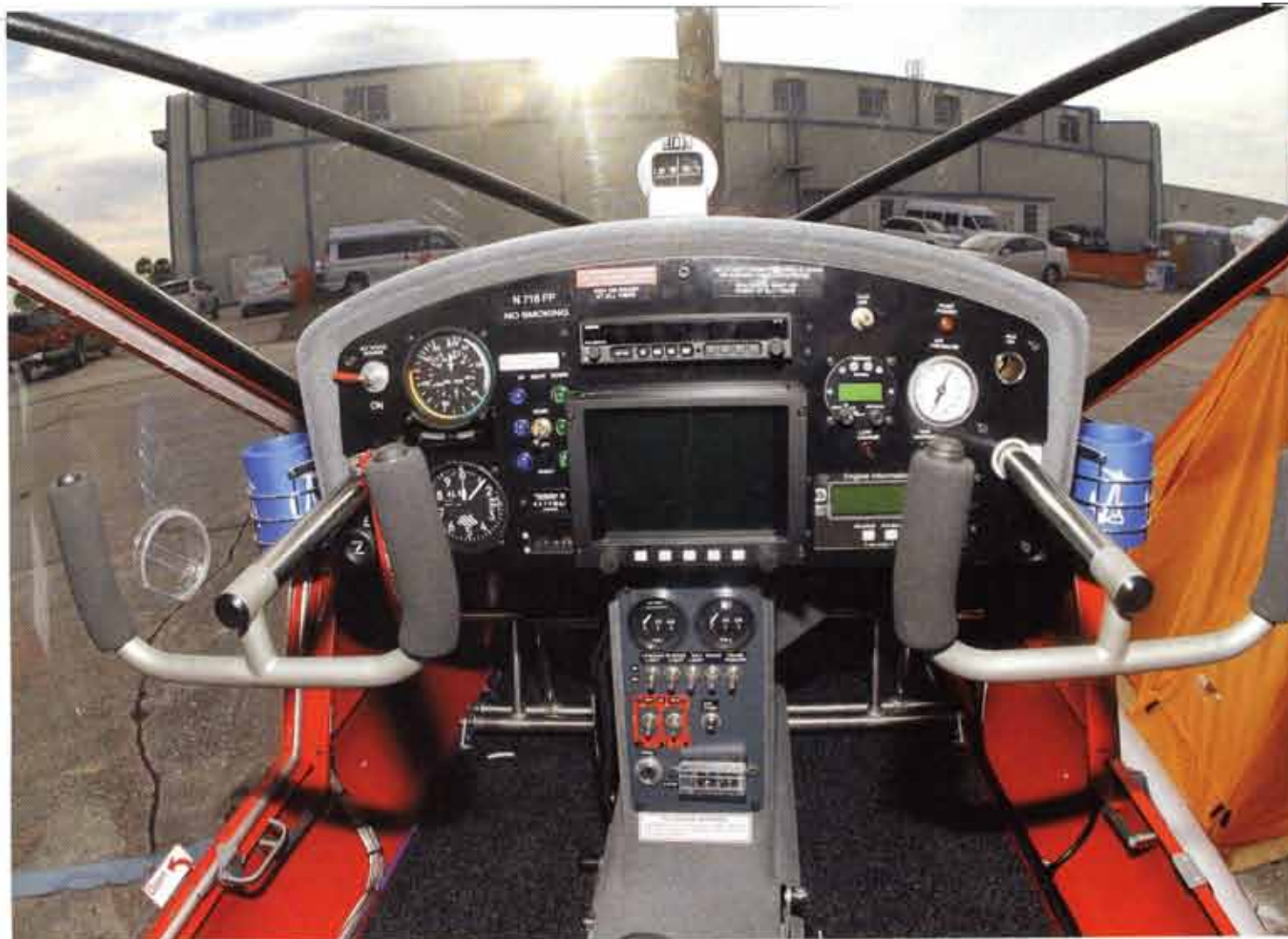
The instrument panel is logically laid out - note the blue and green undercarriage position indicators and the large air pressure gauge.
